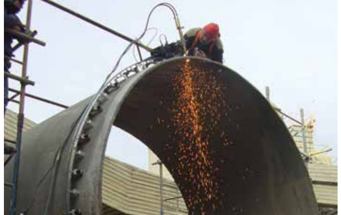
Hi-Flex Rail (FMD) for various circumferential and irregular surface applications down to 30" (760 mm) radius (Page 2)
