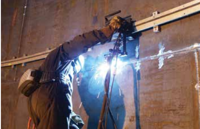
Aluminum Semi-Flex Rail (AFR) for large diameter applications down to a minimum radius of 15' (5 m) (Page 2)
