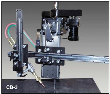
The CB-3 Circle Burner (CBO-3000) uses Oxy-fuel for square or beveled hole cuts (see chart for capacities). Unit includes 2-hose Oxy-fuel machine torch, adjustable tip adaptor, variable speed rotation, vertical and horizontal torch adjustment and rise and fall cam. The CB-3 must be mounted on a column and boom, manipulator or fixture. For more detailed information please see our "CB-3" tech sheet online at bugo.com
