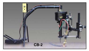
The CB-2 Circle Burner (CBO-2000) uses Oxy-fuel for square or beveled hole cuts (see chart for capacities). The CB-2 is mounted on a special frame with a releasable permanent magnet base. Machine includes variable speed rotation, 2-hose Oxy-fuel machine torch, adjustable tip adaptor, vertical and horizontal torch adjustment and rise and fall cam. For more detailed information please see our "CB-2" tech sheet online at bugo.com
