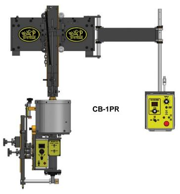
The CB-1PR Plasma Circle Burner with Remote Control (CBP-2020) is designed for cutting beveled holes in lightwall pipe or vessels. This machine is supplied with a Thermal Dynamics air plasma power source (Hypertherm power source also available), torch and 50' (15 m) leads. The CB-1PR must be mounted on a carriage or fixture.
