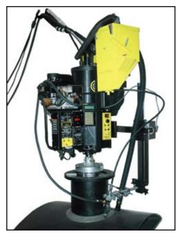
The **CWP-1100 Programmable Circle Welder** is designed for welding of nozzles into vessels utilizing SUB-ARC, MIG or FLUX CORED PROCESS, with gas shielding. The CWP-11 mounts on a 3-Jaw Chuck for welding diameter 6" to 50" (152 to 1270 mm) O.D. Photo shown with optional Flux Recovery System installed.
