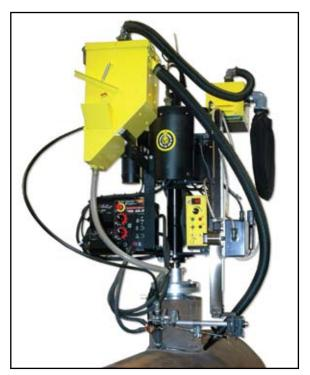
The CWP-1800-SA Programmable Circle Welder is designed for single or multipass welding of couplings or nozzles. This machine uses a microprocessor to control the rise and fall through encoder positioning. Photo shown with optional Flux Recovery System installed.
