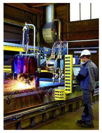
The SUPRAREX<sup>™</sup> HDX is a powerful and extremely durable gantry cutting machine with impressive positioning speed. Its innovative modular system handles a variety of cutting and marking tasks to meet individual application requirements. It can be equipped with tools for cutting, weld edge preparation and marking, and works with plasma, oxy-fuel or both processes in combination.
